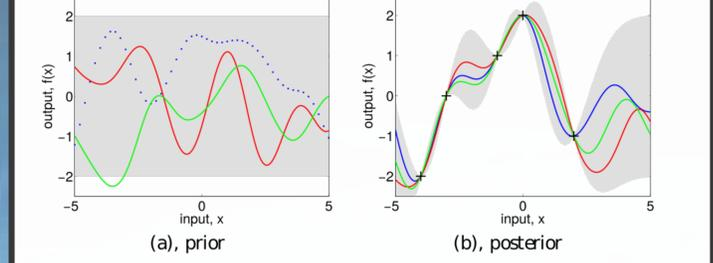
**Figure 3:** Functions drawn from GP prior (a) and posterior (b) i.e. prior conditioned by 5 noiseless data points.[5]
